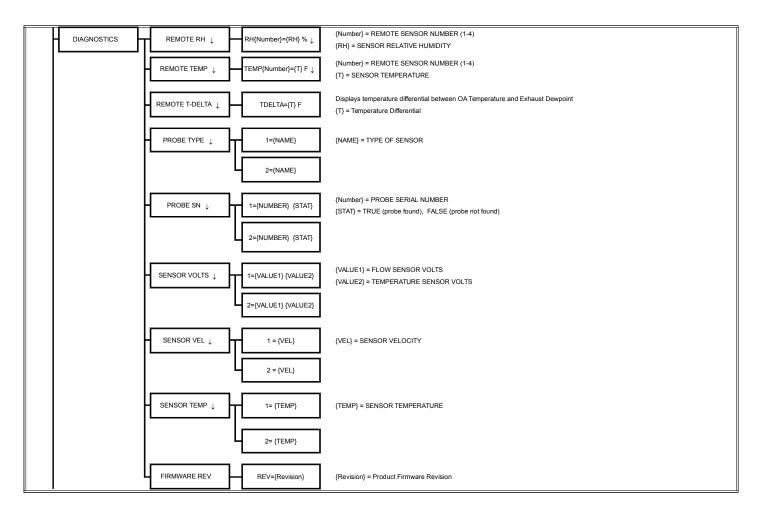
Figure 16. DIAGNOSTICS Menu - Sensor and System Status Menu Detail
