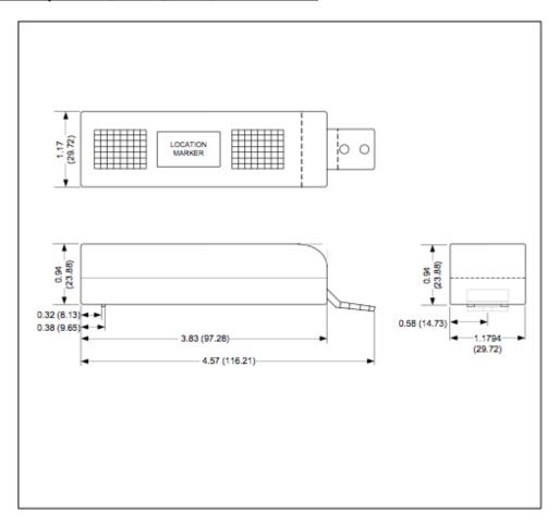
Figure 3. RH/Temperature Sensor Mechanical Detail
