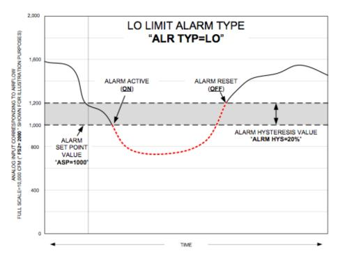
Figure 20. Low Limit Alarm Example
