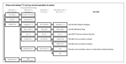
Figure 15. COMM SETUP – RS-485 Communications Setup Menu Detail
