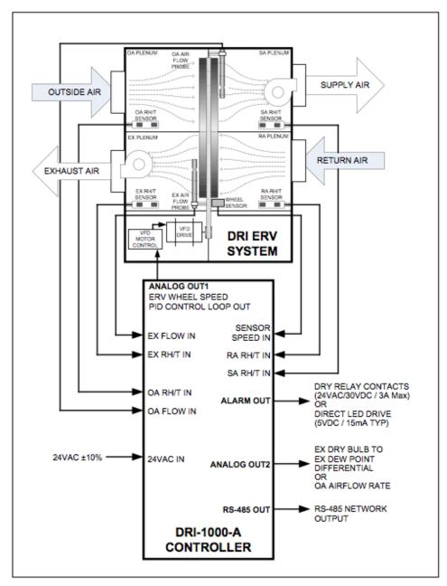
Figure 21. Block Diagram of Typical DRI-1000-A ERV Controller System and DRI ERV System
