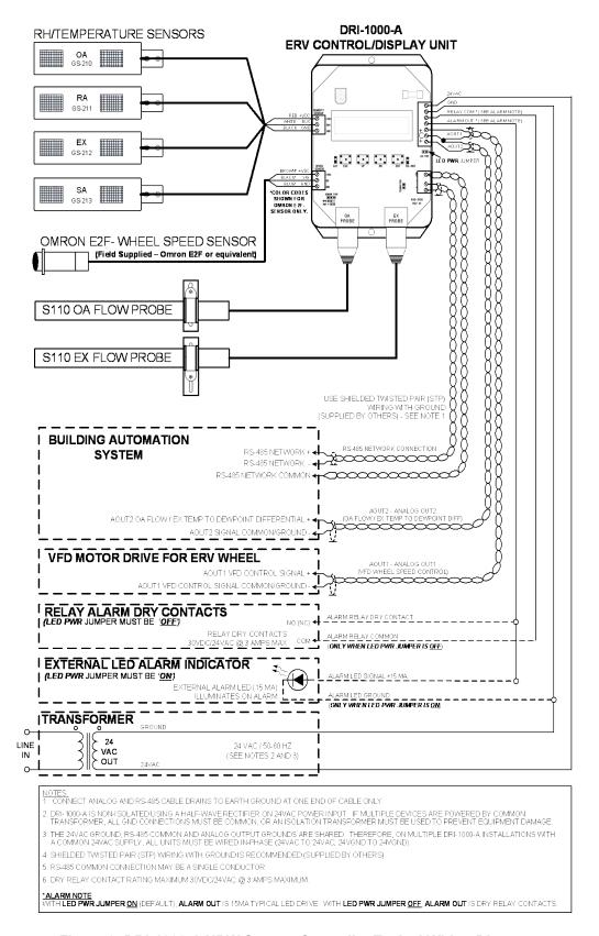
Figure 9. DRI-1000-A HRW System Controller Typical Wiring Diagram
