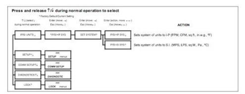
Figure 12. IP/SI UNITS - Units of Measurement Menu Detail
