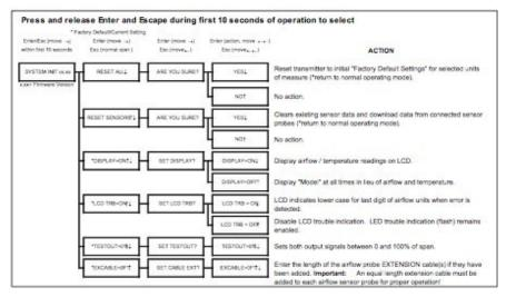
Figure 10. SYSTEM INIT – Initialization Menu Detail
