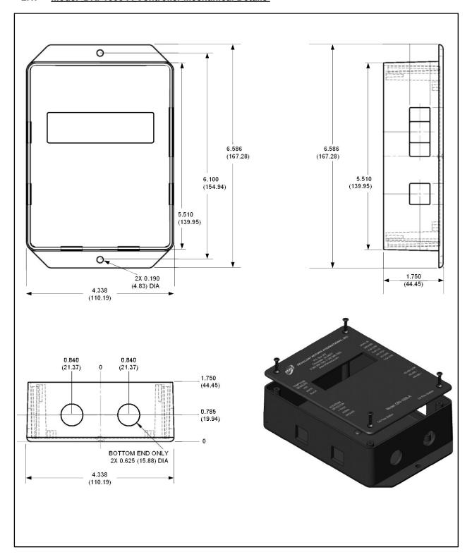
Figure 2. DRI-1000-A Controller/Display Unit Mechanical Detail
