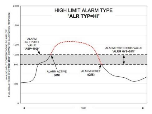
Figure 19. High Limit Alarm Example
