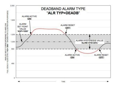
Figure 18. Deadband Alarm Example
