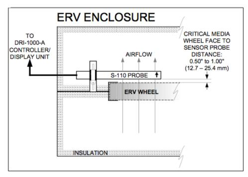
Figure 8. Typical S-110 Airflow Probe Placement Detail
