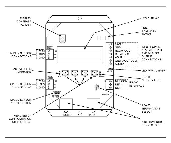
Figure 5. DRI-1000-A Controller/Display Unit Detail View
