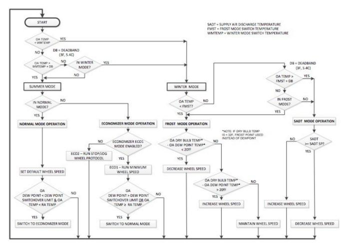
Figure 22: DRI-1000-A Control Logic Flowchart
